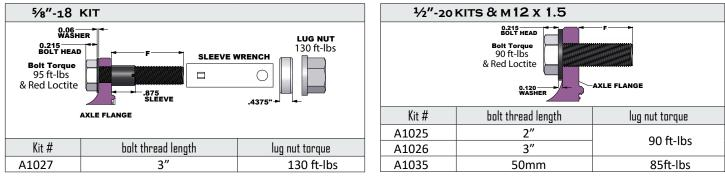
• to calculate length "F" protruding through the axle to mount the rotor and wheel on use the following method:
