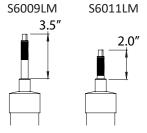
Note: 2005-10 & 2011-14 have different rod shoulder to rod end lengths as shown
