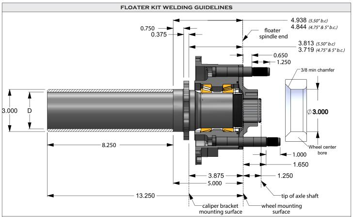
**NOTES:** The 3.000" diameter spindle must be turned to a "D" dimension that's dependents on the particular housing tube inside diameter. See step # 2 for further instructions.
