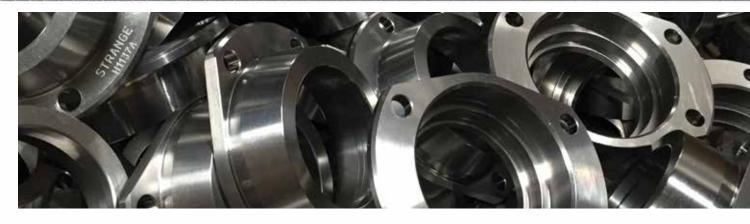
**HOUSING ENDS:** Strange housing ends are machined from MADE IN THE USA forged steel. These premium grade ends are ideal for a new or existing housing that needs to be narrowed. They provide an optimal mounting surface for the brakes to keep in proper alignment with the axle bearing. These housing ends are designed to be easily butt welded with the proper equipment. An alignment bar is
