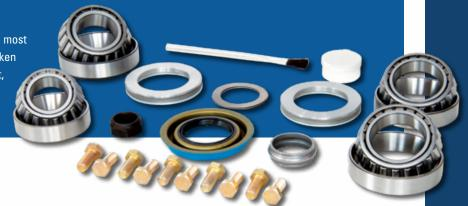
**STRANGE BASIC INSTALLATION KITS:** Basic kits include ring gear bolts, shims, seal, pinion nut, gasket or sealer, brush, marking compound, and crush collar if required. Bearings and races are not included.
