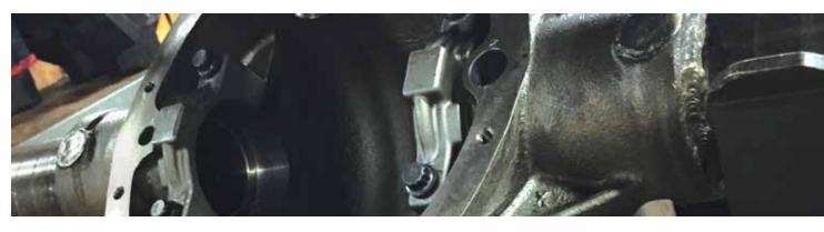
**BARE CASTING:** The Strange 12 bolt casting is much stronger than the 0EM 12 bolt, while still accepting the same components. The casting is poured from proprietary nodular iron which is substantially stronger than cast iron. The main caps are constructed from forged chrome moly instead of cast iron like the originals. These improvements in materials have allowed the casting to be made not only thinner and
