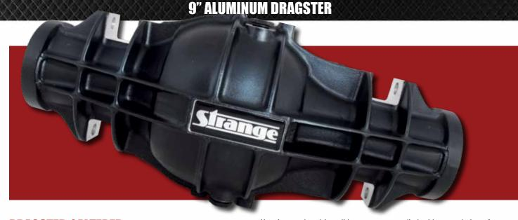
**DRAGSTER / ALTERED:** These housings are available in 26" or 27" widths with the pinion in the center. The 26" housing using Olds brake offset axles would result in 31.664" bare axle flange to axle flange, while the 27" would provide a 32.664" width. The 26" housing using special brake brackets would allow use of axles with an Early Big Ford offset of 2.332", achieving 30.664" bare axle flange to flange. Add your rotor hat thickness to determine your final wheel to wheel.
