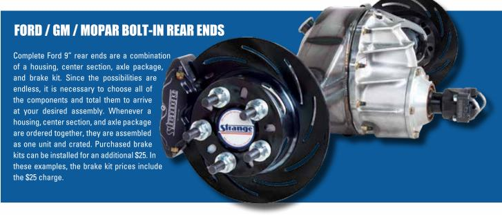
Listed are samples of possible combinations. Options for housing, center section, axle package, and brake kit, are listed within their respective sections.
