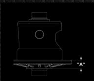
2 series carrier- A= .600" (OEM 2.76-down) 3 series carrier- A= 1.00" (OEM 3.07-3.73) 4 series carrier- A= 1.315" (OEM 4.11-up)
