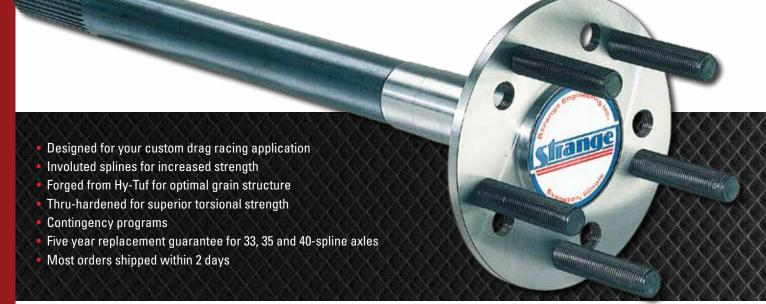
**STRANGE PRO RACE AXLES** are forged from Hy-Tuf alloy steel that was originally developed for highly stressed landing gear in military aircrafts. The material is in the class of Ultra Strength alloys and contains low carbon, high manganese, high nickel, and high molybdenum steel. Pro racing axles are thru-hardened allowing for a Drag Racing shaft with an exceptionally high, 240,000 PSI, tensile strength while retaining ductility.
