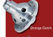
with tapered bores and the side gears have a mating cone shape on their backside. There is a spring or springs that apply pressure to the side gears causing them to wedge into the case. It also uses spider gears and a cross shaft as above. The operation is much the same as the
