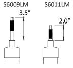
Note: 2005-10 & 2011+ have different rod shoulder to rod end lengths as shown
