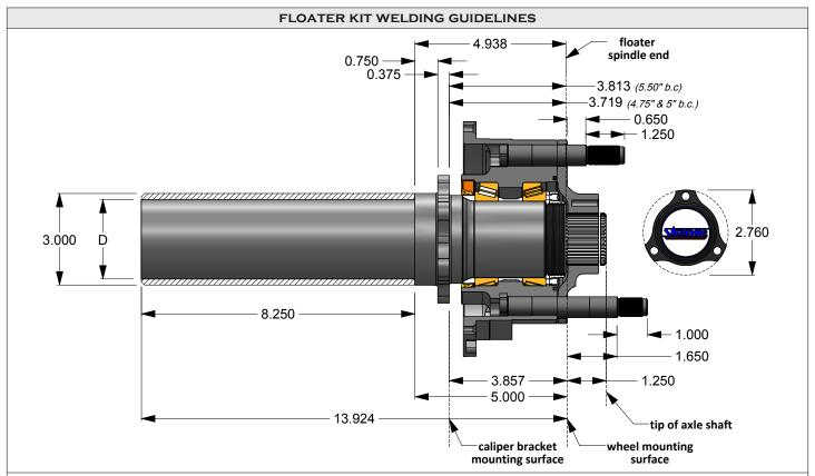
**NOTES:** The 3.000" diameter spindle must be turned to a "D" dimension that's dependents on the particular housing tube inside diameter. See step # 2 for further instructions.
