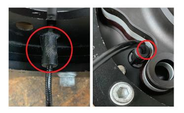
Sensor ribs and body in contact with the spindle flange must be ground away for clearance
