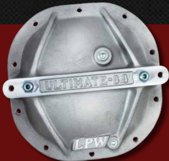
LPW HD aluminum cover ready for back-brace
